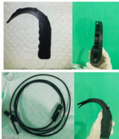
Figure 2. 3D-printed video laryngoscope assembled with an endoscopy camera.
